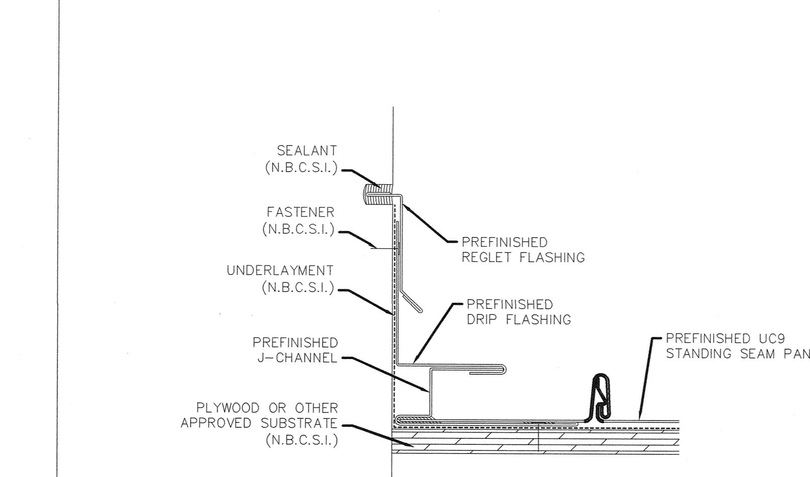
**A4** METAL ROOF RAKE DETAIL
