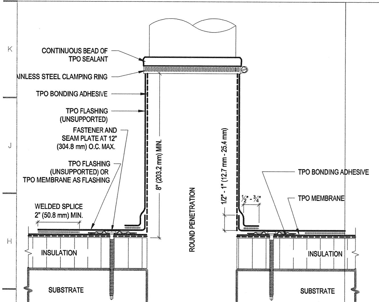
**F1** FIELD FABRICATED PIPE SEAL
